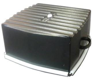
contains a pre-amplifier which is powered directly from the terraTEM console. The TRC sensors are designed to provide an equivalent reception to that of a 1000 square metre single turn receiver loop by compensating for their much reduced area with multiple turns of wire plus electronic pre-amplification.
